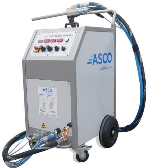
The **ASCOJET 2008 Combi Pro** combines a powerful double hose system, which can be optionally used as a one-hose system, with the option of cleaning with dry ice pellets and the additional abrasive effect of an additive. Thus, users can choose from two blasting options, namely pure dry ice blasting or combination blasting.
