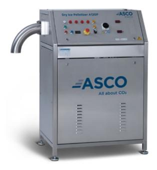
The **ASCO** Dry Ice Pelletizer A120P is a compact, powerful and versatile machine producing high quality dry ice pellets in five different sizes (1.7, 3, 6, 10 and 16 mm) (1/16, 1/8, 1/4 and 5/8 in). Having a production capacity of 120 kg/h (264.55 lb/h) this dry ice machine guarantees quality and flexibility in the daily working process.
