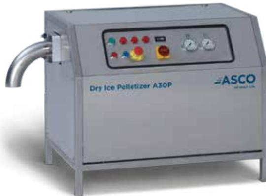
The **ASCO** Dry Ice Pelletizer A30P having a production capacity of 30 kg per hour (66.14 lb/h) is suitable for the production of small amounts of dry ice for cooling purposes.
