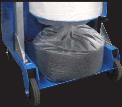
The discharge flap discharges the suction material into the MultiPac collection bag. The MultiPac bag is then closed off with two hose clamps. By cutting off the sealed part of the bag the suction material can be disposed of without dust propagation. The MultiPac collection bag is long enough for 50 to 60 bagging units.
