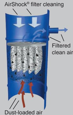
The AirShock® inflates the filter pockets instantaneously. Accumulated dust drops off and falls down into the collection container.
