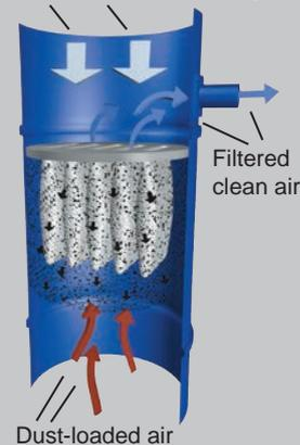
The AirShock® inflates the filter pockets instantaneously. Accumulated dust drops off and falls down into the collection container.
