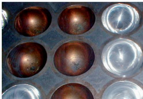
Mould for the production of tennis balls
