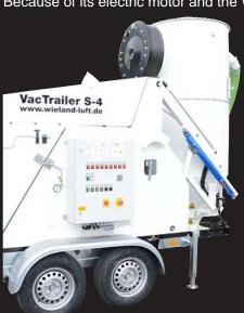
system, the unit is certified according to Atex 3D and can be operated inside zone 22. If a Diesel operated unit is required, the S-4 can still safely extract explosive suction material but must remain outside zone 22 - not a problem, taken into account that due to the suction power of the S-4 a suction line of 100 m or more is easily possible!
