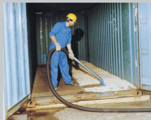
Container cleaning with mobile and stationary vacuum systems
